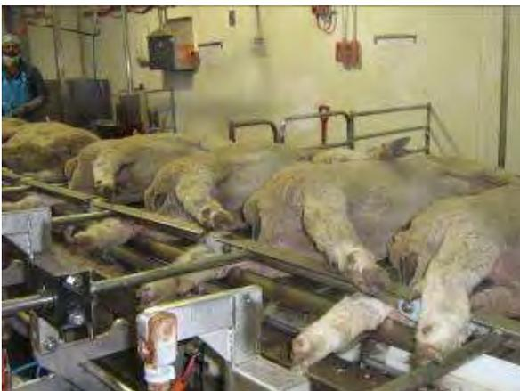
**Figure 1.** High frequency immobilisation used immediately post exsanguination and before the carcasses are placed on the chain.
