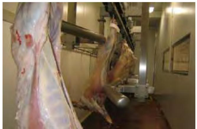
**Figure 4.** Post-dressing medium voltage electrical stimulation unit, bottom rail is active.
