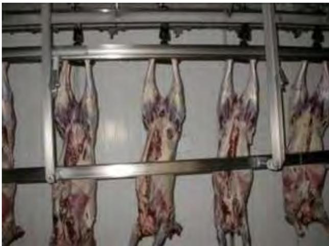
**Figure 3.** High voltage electrical stimulation unit, bottom rail is active.
