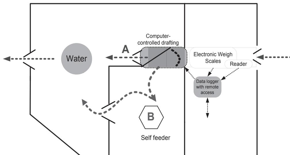
**Fig. 1.** Components of a precision nutrition system. Animals enter through spear gates on right-hand side and are identified by electronic tags as they walk over the weighing platform. From the weighing platform, sheep are either drafted into the area containing the self-feeder (B) or allowed to pass through to water (A). Spear gates maintain a uni-directional flow with access to feed controlled by computer-directed drafting.
