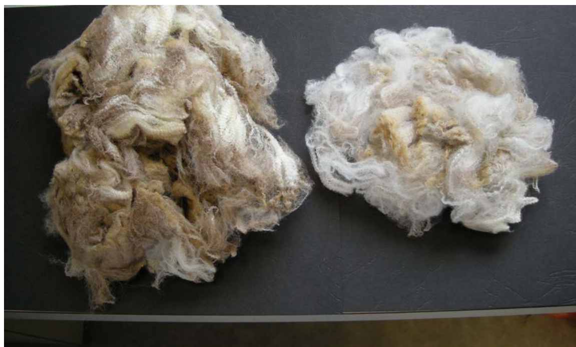
Figure 6: Turretfield mid-side sample before solvent scouring (left) and after a dichloromethane Soxtherm solvent extraction
