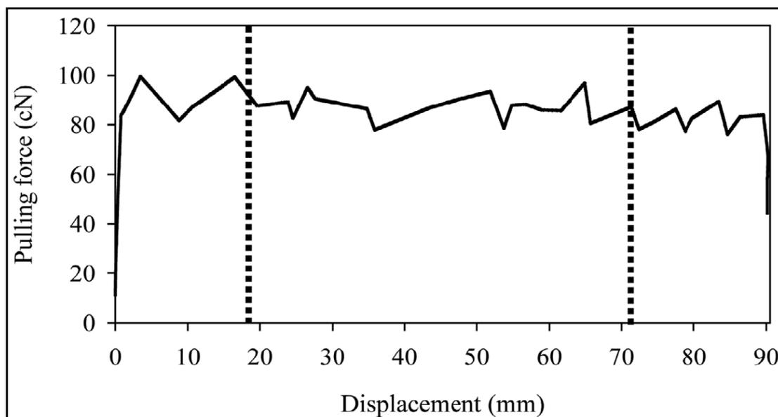
Figure 17. A typical pulling force curve of a fabric (Zhang et al., 2005)
