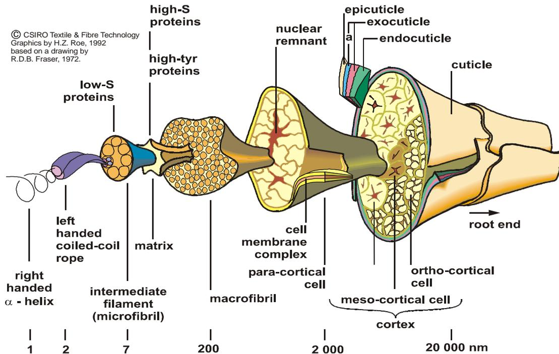
Figure 19. Schematic diagram of the structure of a wool fibre (Kirk-Othmer, 1998)
