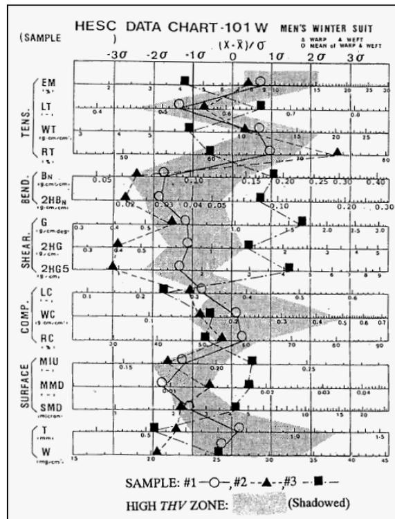
Figure 7. Application of KESF testing to process control (Kawabata and Niwa, 1996): KESF parameters for 3 samples and the zone of parameters for high THV fabrics.
