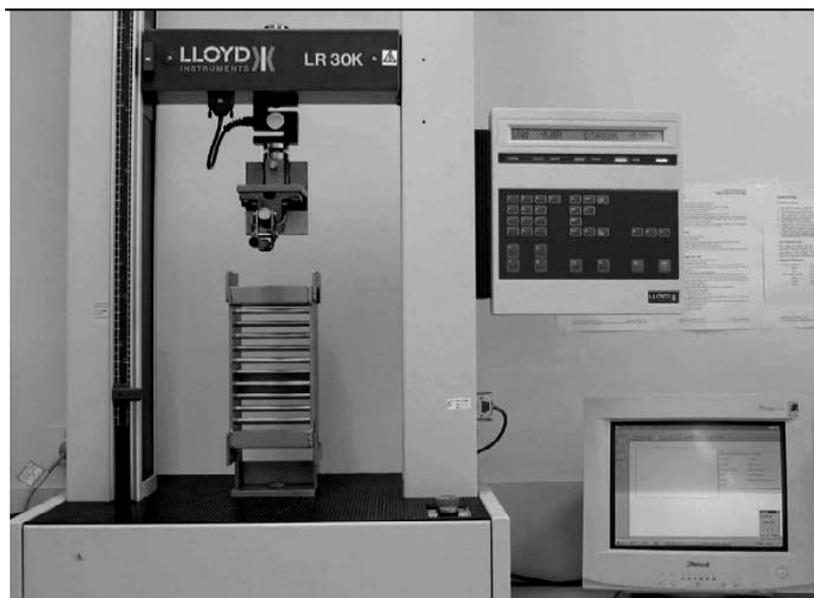
Figure 16. A Pulling Force Method for the evaluation of fabric softness (Zhang et al., 2005)
