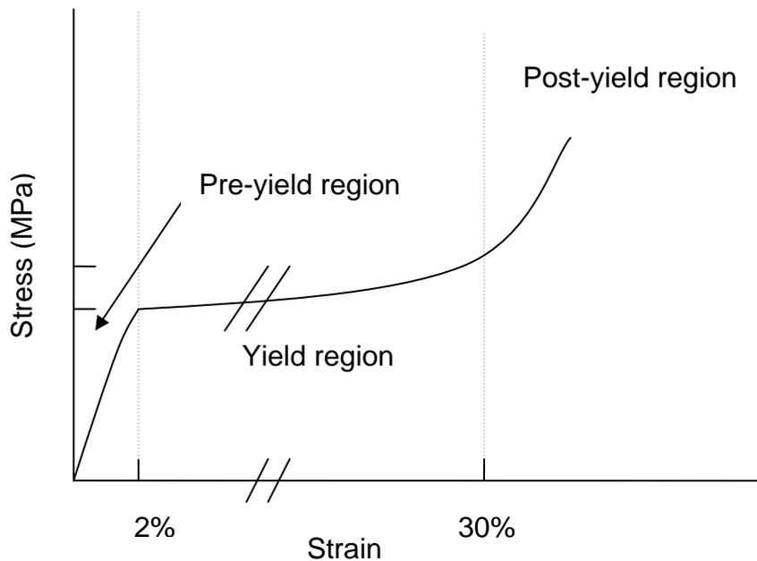
Figure 22. Schematic of a typical stress-strain curve for a wool fibre in water at 20°C (not drawn to scale)
