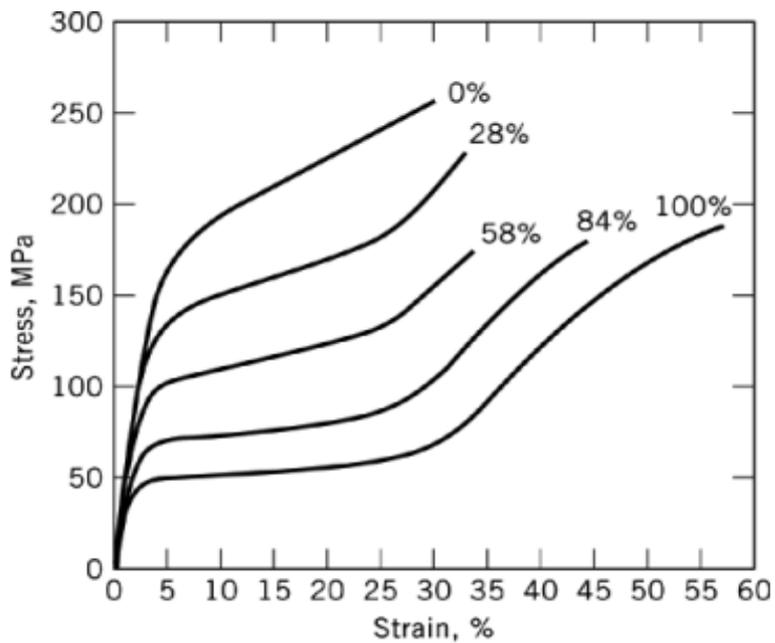
Figure 21. The stress-strain curves of a wool fibre at different relative humidities (Reproduced from the Kirk-Othmer "Encyclopaedia of Chemical Technology", 1998, (Postle et al., 1988))
