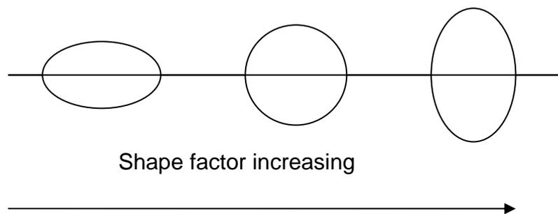
Figure 23. Relationship fibre shape and shape factor
