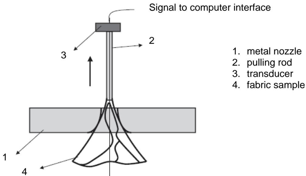
Figure 14. The technique of PhabrOmeter (Pan 2006)
