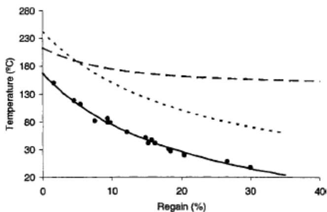
Figure 24. Glass-transition (—) (Wortmann et al., 1984), indicative minimum permanent setting temperature (----) and melting temperature (---) of wool as a function of regain (Feughelman, 1989) (Reproduced from the Kirk-Othmer “Encyclopaedia of Chemical Technology”, 1998, (Postle et al., 1988)
