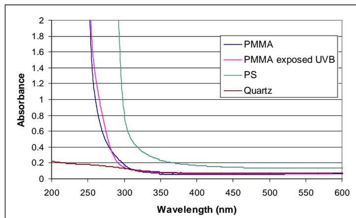
**Figure 2** Absorbance of quartz, polystyrene and PMMA cuvettes
