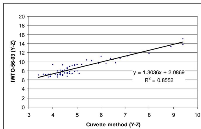
**Figure 3** Yellowness (Y-Z) of wool measured in cuvettes and by IWTO-56-03 test method
