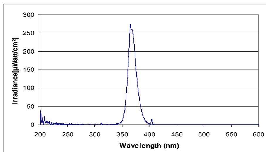
**Figure 7** Spectral intensity of Philips TUV (UVA) lamp
