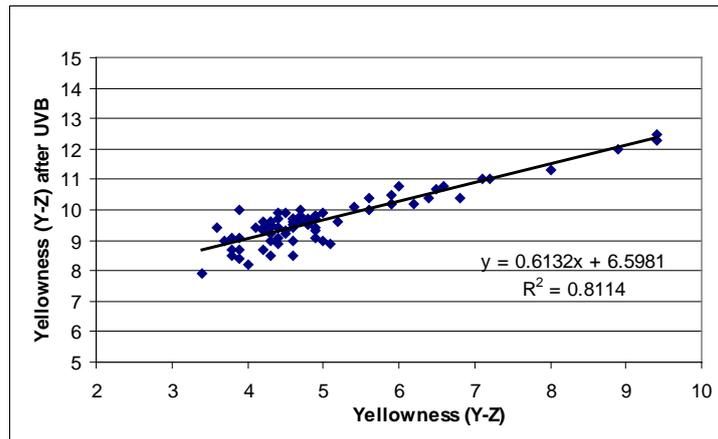
**Figure 5** Yellowness (Y-Z) of IN flock samples measured in cuvettes before and after exposure to UVB for four hours
