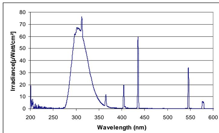
**Figure 4** Spectral intensity of Philips TL20W/12RS (UVB) lamp
