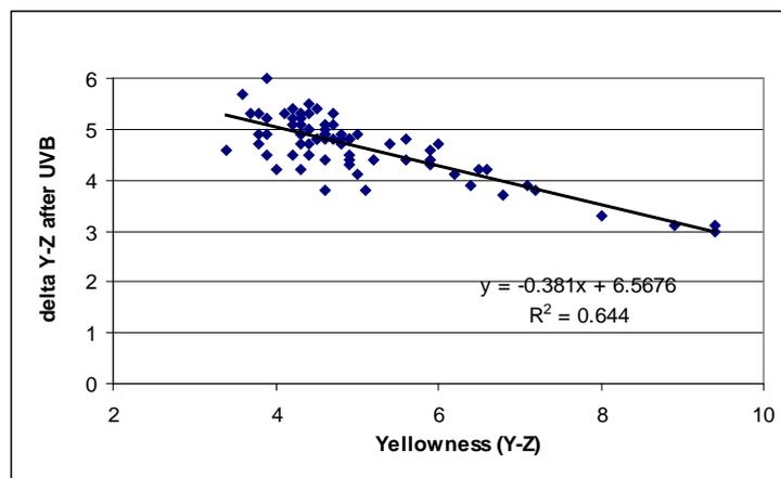
**Figure 6** Yellowness (Y-Z) of IN flock samples measured in cuvettes before exposure and the change in yellowness after exposure to UVB for four hours
