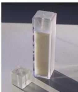
**Figure 1** packed cuvette and Perspex cap
