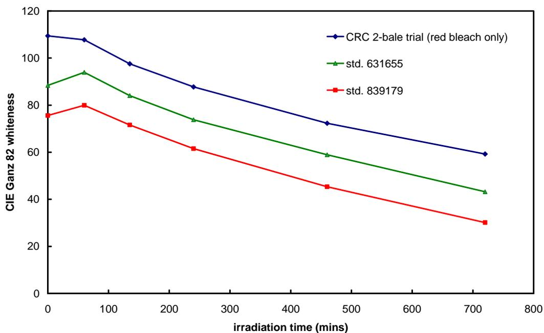
**Figure 7 Dry photoyellowing of finished Toi Toi knitted fabrics with simulated sunlight**
