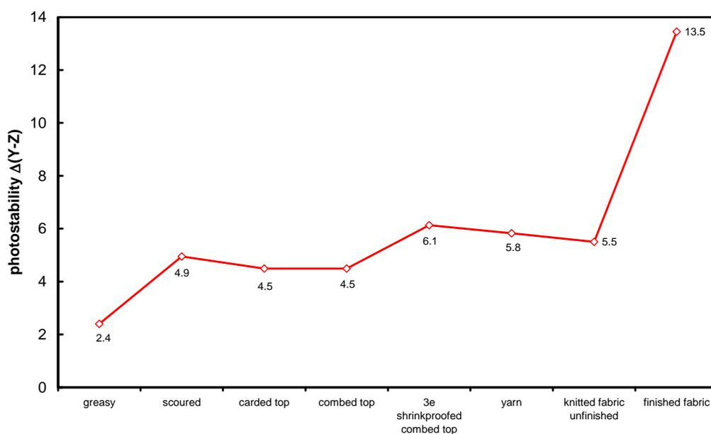
**Figure 6 Changes in photostability  $\Delta(Y-Z)$  during processing measured using the CSIRO small sample method**
