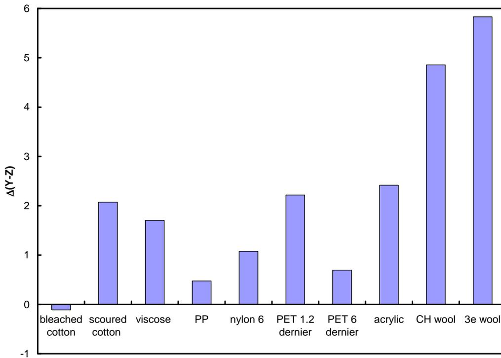
**Figure 9 Photostability  $\Delta(Y-Z)$  of different fibres measured using the CSIRO small sample method**
