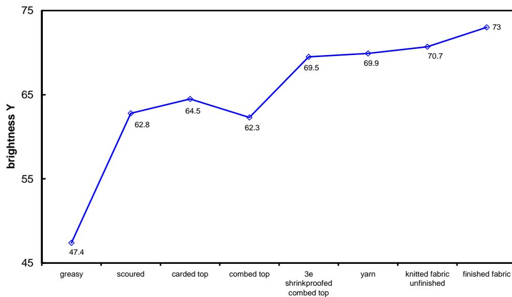
**Figure 5 Changes in fibre brightness (Y) during processing measured using the CSIRO small sample method**
