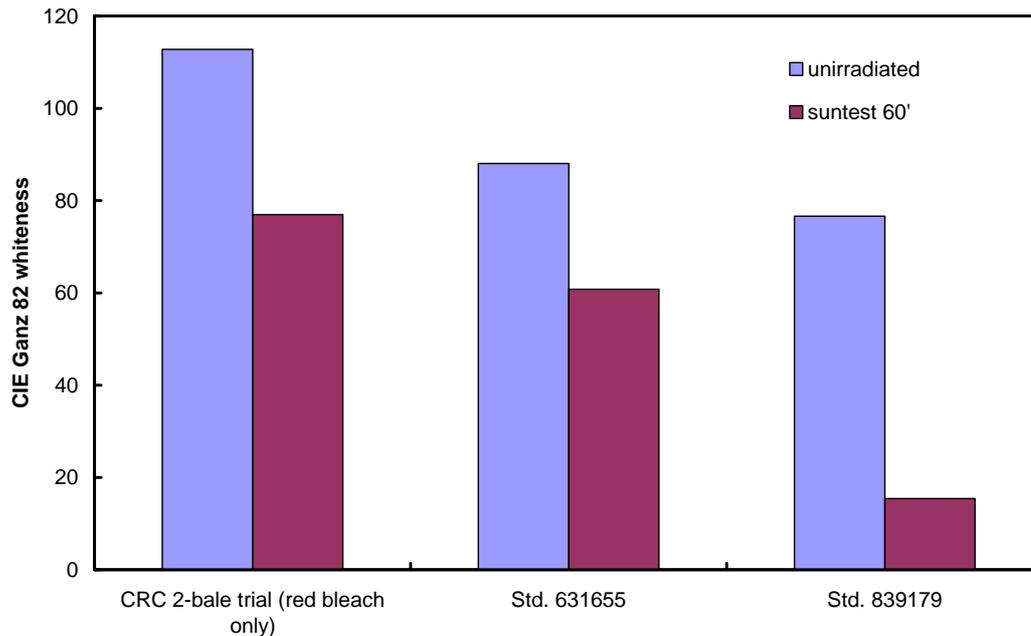
**Figure 8 Wet photoyellowing of finished Toi Toi fabrics with simulated sunlight**
