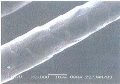
**Traditional shrink-proof technology:** Chlorine (erode the scale) & Resin
