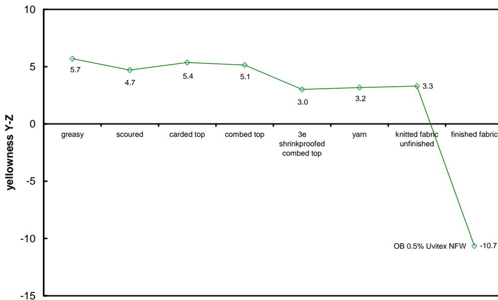
**Figure 4 Changes in fibre yellowness (Y-Z) during processing measured using CSIRO small sample method**
