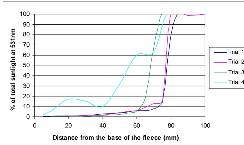
**Figure 4** Penetration of sunlight through a simulated Merino fleece
