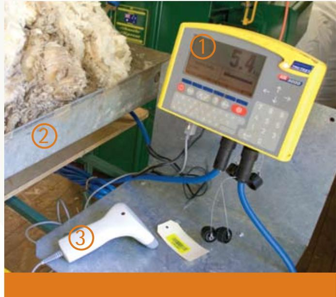
Image 1. Tru-Test indicator and barcode scanner
